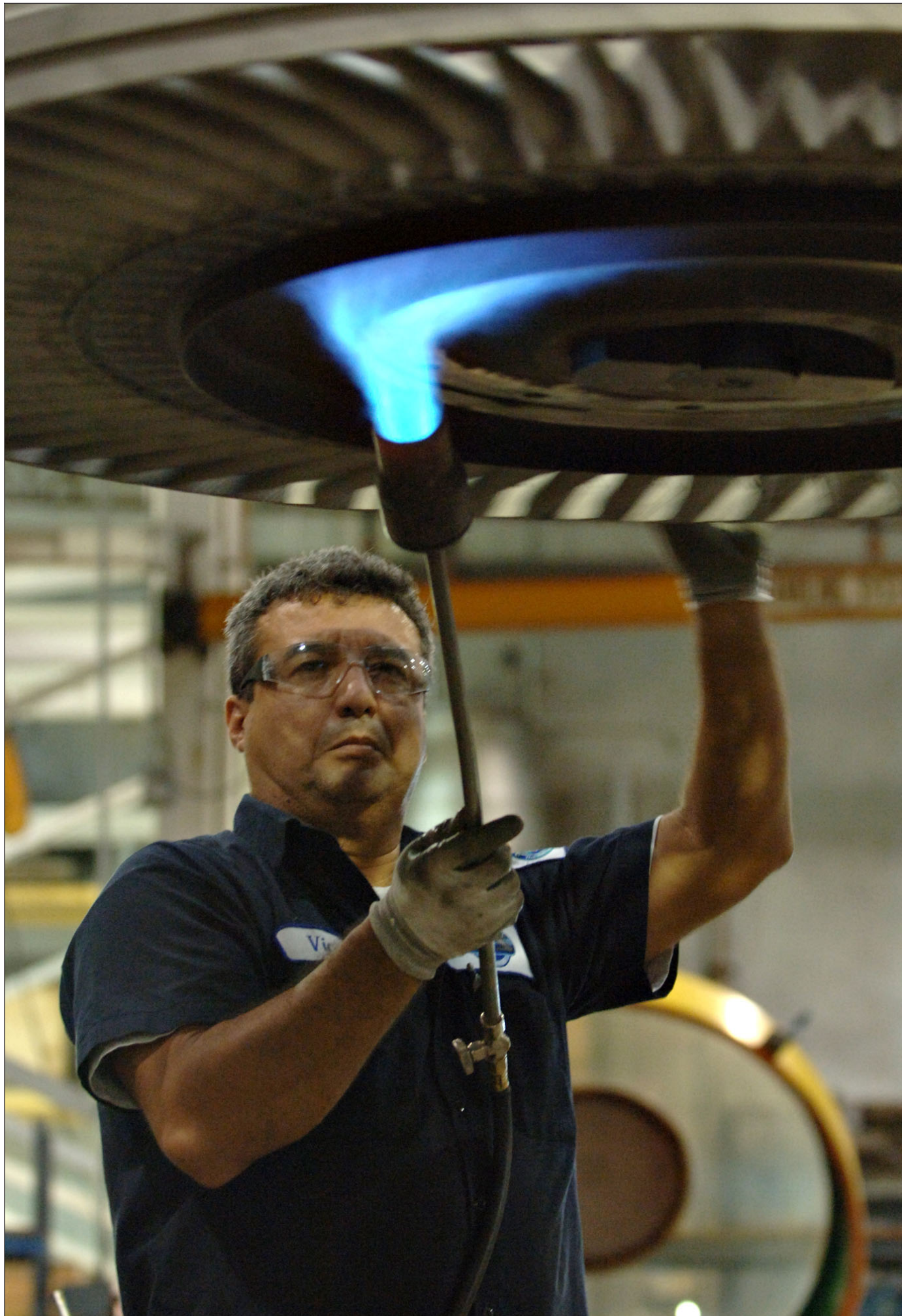
FITTING IN AT FAU: Victor Salazar of Boca Raton heats up a turbine to be fitted onto a hub at Jet Turbine Service's facility in FAU's research and development park in Boca Raton. At FAU, Jet Turbine turns former aircraft jet engines into power generation units for ground and marine uses. Staff photo/Jim Rassol
