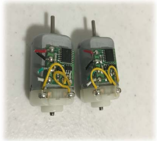
Figure 5. Servo Motor Controller Modification (Proprietary Control Boards Shown)
