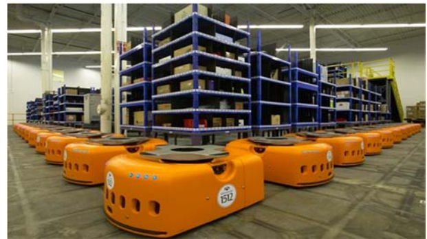
Figure 1. Amazon warehouse automated guided vehicles (AGV)
