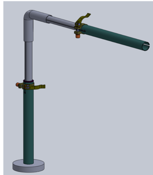
Figure 1. Adjustable cylindrical bars for vertical and horizontal motion
