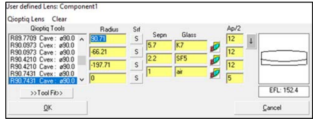
Figure 2. Lens Parameters for Simulation of ROARSAT Optical System
